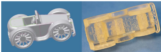
Figure 15: Good model for PR-Car use; tire axle also rotate
